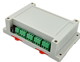
ESP32-C6-EVB Board Support Tasmota 4 Relay 4 Input with WiFi BI
