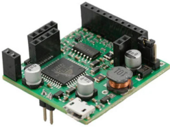
EspoTek Labrador: Easy-to-Use, All-in-One USB Oscilloscopes
