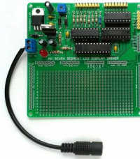
Serial driver for large seven segment LED displays (PCB only)
