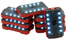
SmartClips, bluetooth nodes with LED lights and sensors for use
