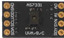
AS7331 UVA/B/C Light Sensor Breakout
