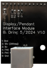
FluidNC RJ12 Pendant/Display Module
