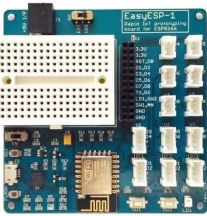
EasyESP-1: An ESP8266 experimenter board for beginners
