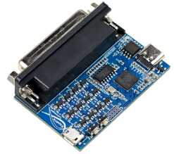
PicoBOB CNC Control Module for GRBLHAL
