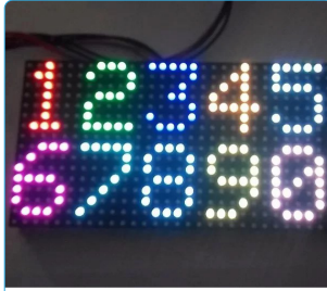
16x32 RGB LED matrix panel + Arduino driver shield
